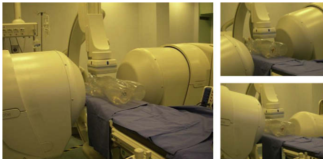
Fig. 2. Robotic magnetic navigation system (Niobe ® model, Stereotaxis Inc., USA) and experimental set-up for testing the manoeuvrability of the magnetically enabled capsule inside a plastic phantom. The phantom was laid on the patient's table, between the two magnets of the system and below the integrated fluoroscopic scanner.
